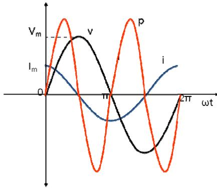
As seen from the power waveform, the instantaneous power is alternately positive and negative. When the power is positive, the power flows from the source to the capacitor and when the power is negative, the power flows from the capacitor to the source. The positive power is equal to the negative power and hence the average power in the circuit is equal to zero. The power just flows between the source and the capacitor, but the capacitor does not consume any power.
