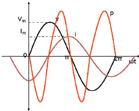
As seen from the power waveform, the instantaneous power is alternately positive and negative. When the power is positive, the power flows from the source to the inductor and when the power is negative, the power flows from the inductor to the source. The positive power is equal to the negative power and hence the average power in the circuit is equal to zero. The power just flows between the source and the inductor, but the inductor does not consume any power.
