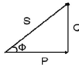
The power triangle is right angled triangle with P and Q as two sides and S as the hypotenuse. The angle between the base and hypotenuse is  $\Phi$ . The power triangle enables us to calculate the following things.
