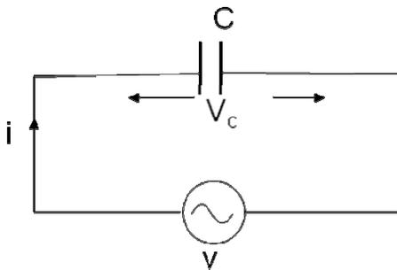
Consider an AC circuit with a pure capacitance  $C$  as shown in the figure. The alternating voltage  $v$  is given by
