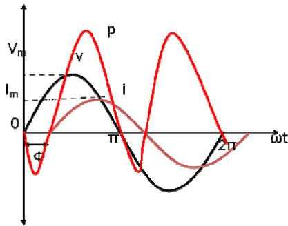
As seen from the power waveform, the instantaneous power is alternately positive and negative. When the power is positive, the power flows from the source to the load and when the power is negative, the power flows from the load to the source. The positive power is not equal to the negative power and hence the average power in the circuit is not equal to zero.
