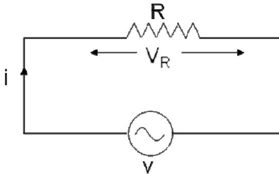
Consider an AC circuit with a pure resistance  $R$  as shown in the figure. The alternating voltage  $v$  is given by
