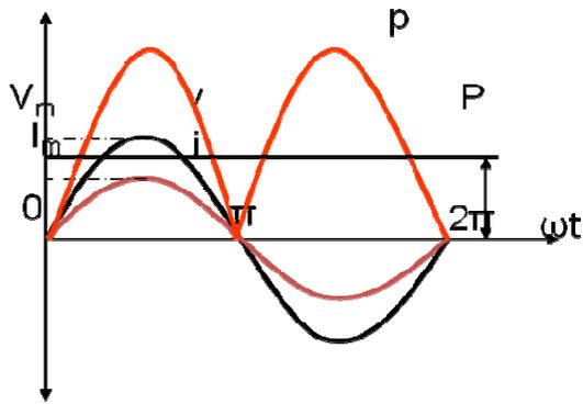
As seen from the waveform, the instantaneous power is always positive meaning that the power always flows from the source to the load.
