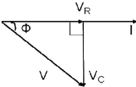
The current  $I$  is taken as the reference phasor. The voltage  $V_R$  is in phase with  $I$  and the voltage  $V_C$  lags behind the current by  $90^\circ$ . The resultant voltage  $V$  can be drawn as shown in the figure. From the phasor diagram we observe that the voltage lags behind the current by an angle  $\Phi$  or in other words the current leads the voltage by an angle  $\Phi$ .
