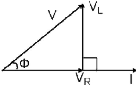
The current  $I$  is taken as the reference phasor. The voltage  $V_R$  is in phase with  $I$  and the voltage  $V_L$  leads the current by  $90^\circ$ . The resultant voltage  $V$  can be drawn as shown in the figure. From the phasor diagram we observe that the voltage leads the current by an angle  $\Phi$  or in other words the current lags behind the voltage by an angle  $\Phi$ .
