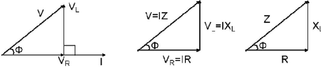
The impedance triangle is right angled triangle with  $R$  and  $X_L$  as two sides and impedance as the hypotenuse. The angle between the base and hypotenuse is  $\Phi$ . The impedance triangle enables us to calculate the following things.
