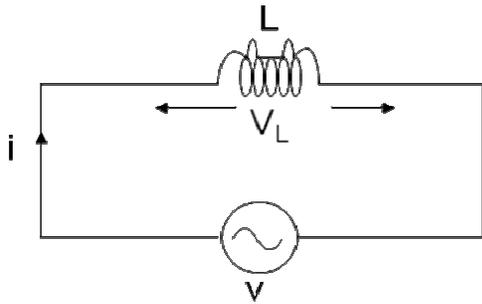
Consider an AC circuit with a pure inductance  $L$  as shown in the figure. The alternating voltage  $v$  is given by
